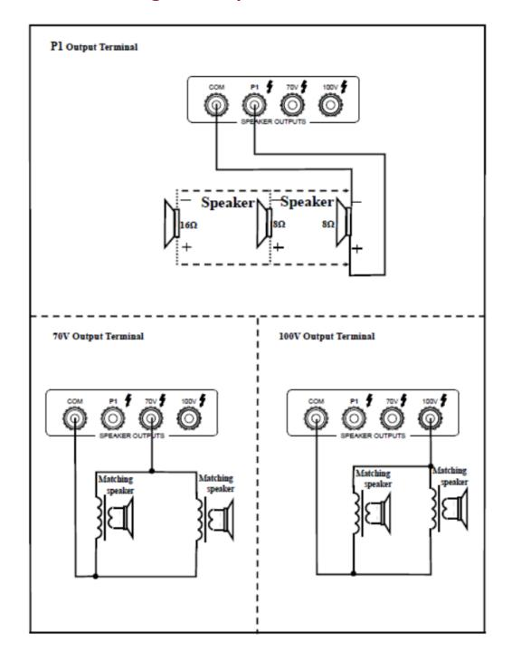
Note: The four outputs are connected using the following methods: COM-P1, COM-70V, and COM-100V. Only one set of output terminals can be connected, and the
